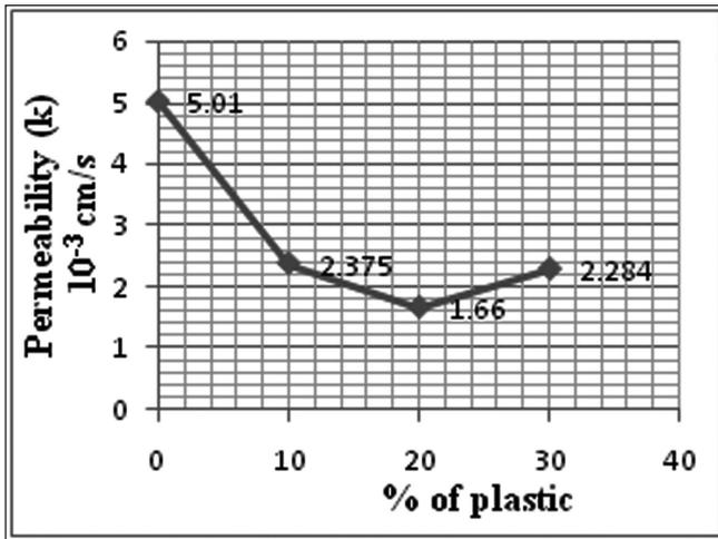
Fig 3: Permeability of mixture for different % of plastic
