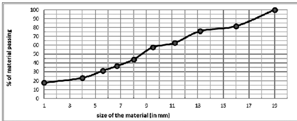
Figure 3. The above figure is showing the size distribution of the sieved material
