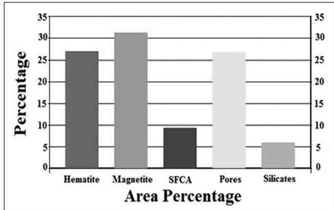
Fig. 4: Graphical analysis of different phases of optimize sample
