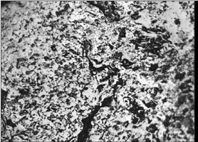
Fig. 3: Microstructure of optimize sinter
