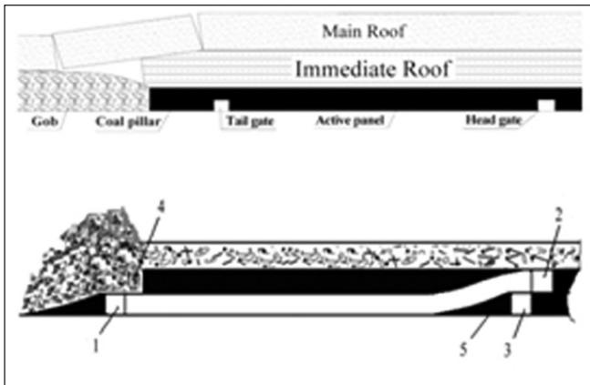
Fig.9. Typical LMSG top coal caving (Wang et al., 2017)
