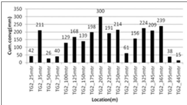
Fig.8. Maximum cumulative convergence in tailgate (TG2) of Adriyala Longwall Panel-2
