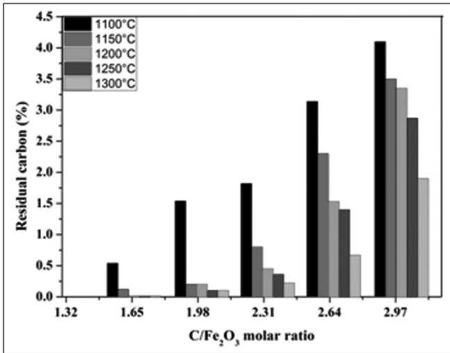
Fig. 3 Variation of residual carbon content in the reduced pellets at different carbon contents at different temperatures
