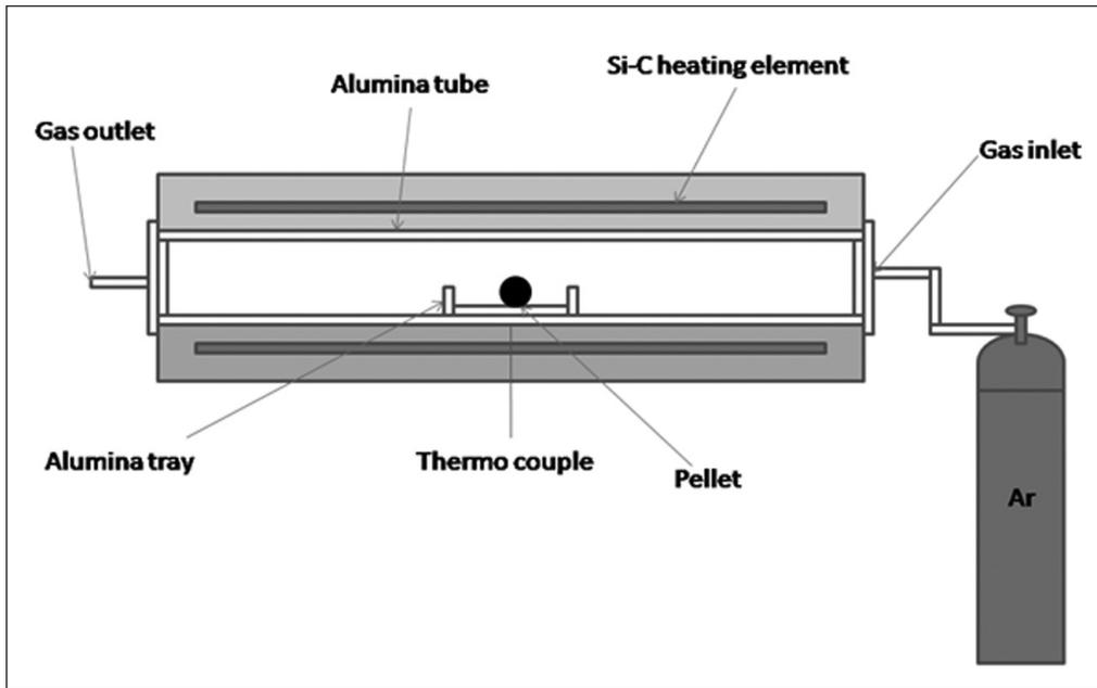
*Fig. 1 Schematic representation of the experimental set up*
