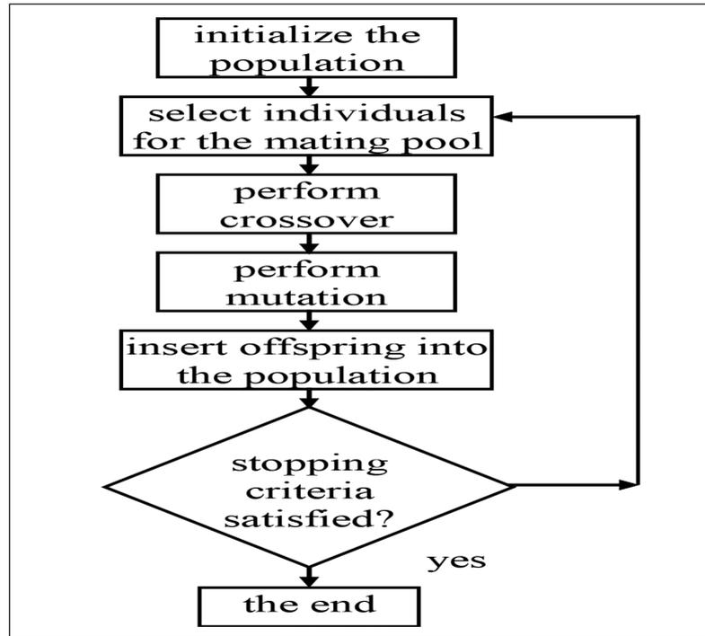
Fig.2: Flowchart of a genetic algorithm
