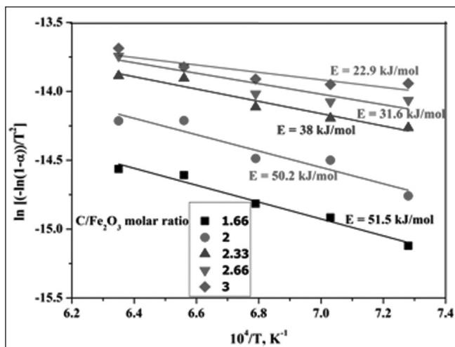
Fig. 5 Coats-Redfern plot of non-isothermal reduction data for different carbon containing pellets
