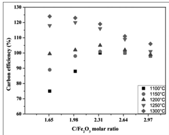
Fig. 4 Variation of Carbon Efficiency with temperature and carbon content
