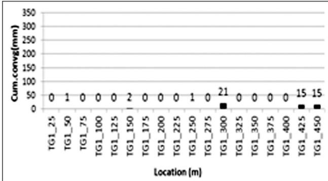
Fig.7. Maximum cumulative convergence in tailgate (TG1) of Adriyala Longwall Panel-1
