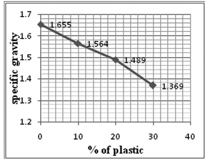
Fig 2: Specific gravity of BA and plastic mixtures for different percentages of plastic
