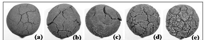
Fig. 7 Surface morphology of the reduced pellets for C/Fe<sub>2</sub>O<sub>3</sub> molar ratio of 3 at different temperature (a) 1100, (b) 1150, (c) 1200, (d) 1250, and (e) 1300°C
