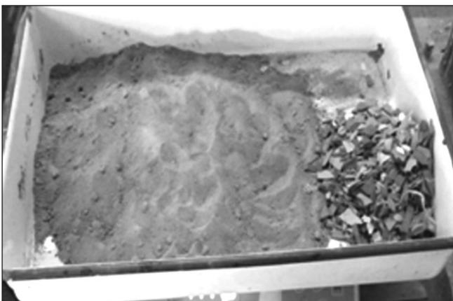
Fig 1: Bottom ash and plastic chips
