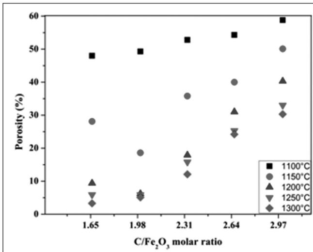
Fig. 8 Effect of temperature and carbon content on porosity of the reduced pellets
