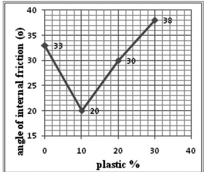
Fig 6: Angle of Internal Friction for different % of plastic
