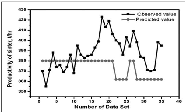
*Fig. 1: Plot of predicted and the corresponding observed productivity of sinter as a function of no. of data sets for testing*
