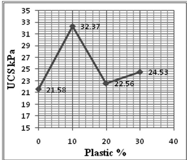
Fig 4: Uniaxial compressive strength for different % of plastic
