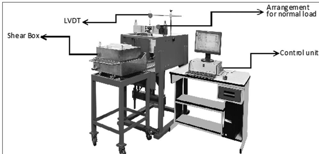
Figure 2. Setup of direct shear testing machine of 30 cm × 30 cm shear box size
