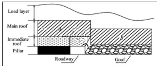
Fig.10. Schematic of RSBT method (Tao et al., 2018)
