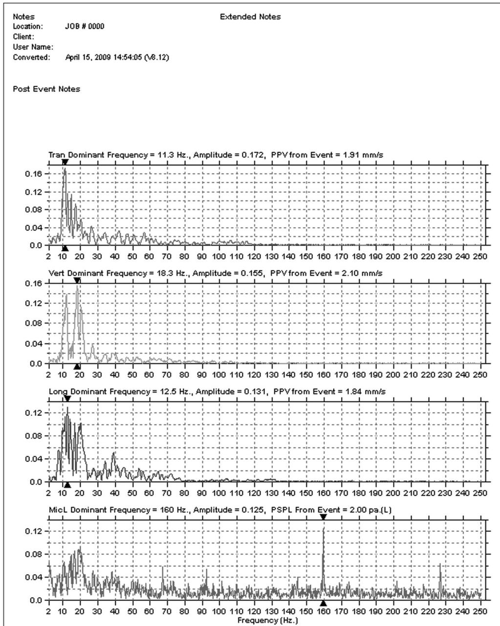
Fig 4: Wave pattern in a typical blast vibration data-Case study-2
