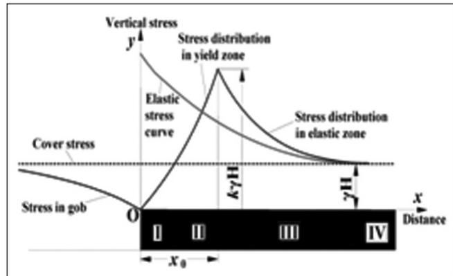
Fig.5. Side stress profile in longwall panel (Suchowerska, 2013).
