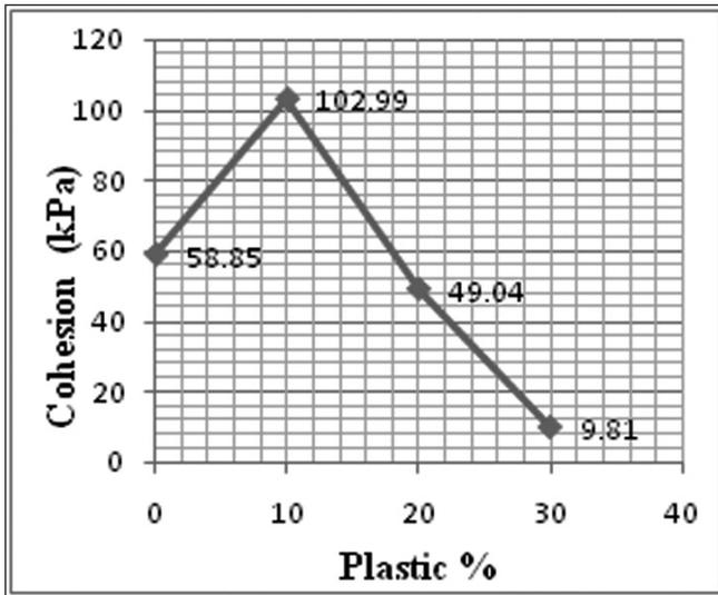
Fig 5: Cohesion for different % of plastic
