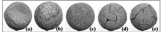
Fig. 6 Surface morphology of the reduced pellets at 1150°C for different C/Fe<sub>2</sub>O<sub>3</sub> molar ratios (a) 1.66, (b) 2, (c) 2.33, (d) 2.66, and (e) 3
