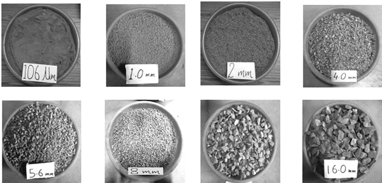
Figure 1. Different sizes of the material mix after sieving obtained from overburden dump
