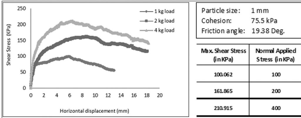
Figure 4. Example plot of shear stress (in kPa) vs horizontal displacement (in mm)
