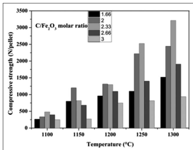
Fig. 9 Compressive strength of the reduced pellets as a function of temperature and carbon content
