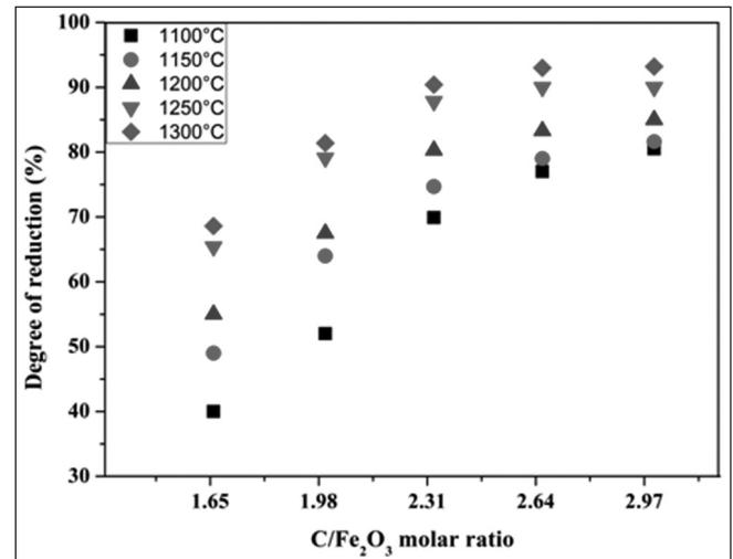
Fig. 2 Effect of temperature and carbon content on degree of reduction
