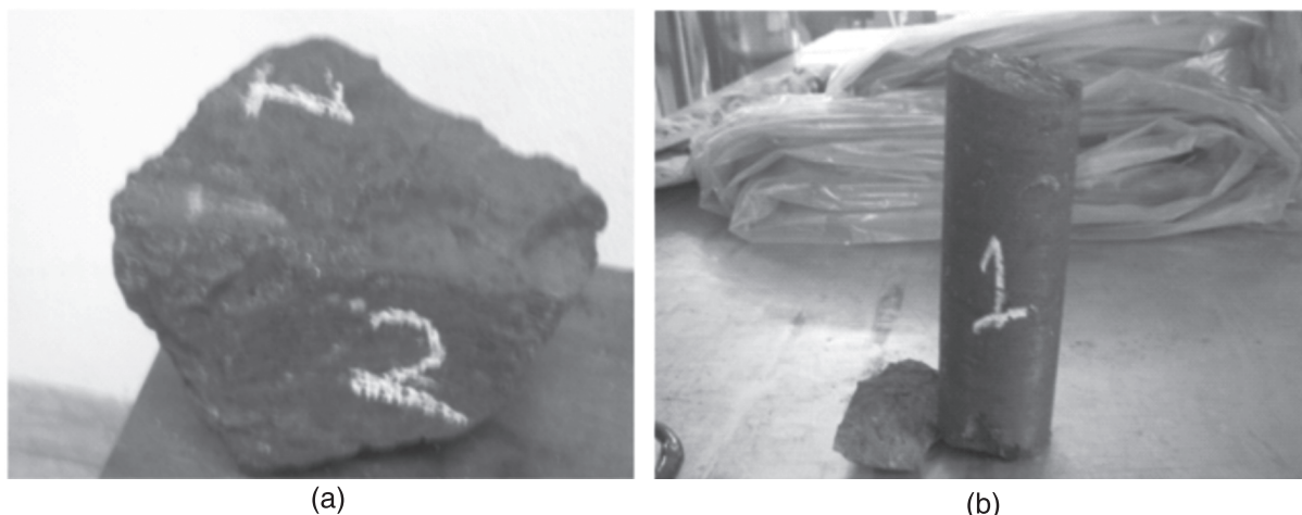
Figure 6. (a) Sample coal block with directions 1 & 2; (b). Core obtained from the sample coal in the direction 1
