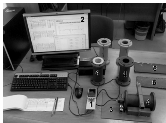
Fig. 2 General view of the measurement setup: 1 - profilometer, 2 - PC, 3 - lodgment, 4 - prototypes with a polyurethane coating, 5 - element of the steel pipe (new pipe), 6 - element of a steel pipe with a run-roughness (trumpet, the former in operation)
